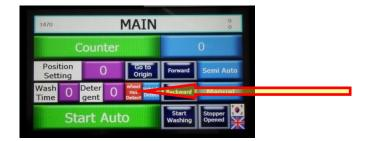
Operation of the product is normal when the background color of "Wheel Not Detect" button pointed by an arrow is in red, but it is not when it turns to blue.
