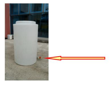
Dilute the detergent provided by us with water in the ratio of 1 to 2 and open the valve at the bottom of the detergent tank at 45 degrees.
