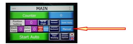
Touch "Manual" button as pointed by an arrow mark and the screen will be changed as shown below
