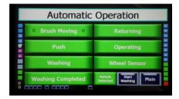
Automatic Operation screen shows the progress of the operation according to the sequence of work flow in order of, from the top left side, "Brush Moving", "Push", "Washing", "Washing Completed" and "Returning". And the operation status can be also monitoredaccording to the background color of "Operating" button on the right(Red means normal operation) and "Wheel Sensor" button will display "Wheel Not Detect" when a failure occurs.
